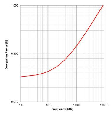
Test Equipment: E4991A or equivalent
