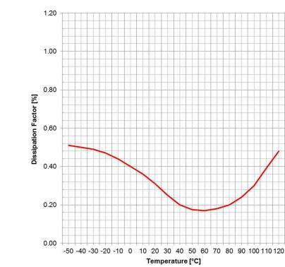
Test Equipment: E4991A or equivalent
