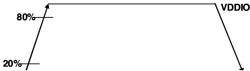
Figure 4. Output Pad Transition Waveform
