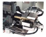
The combination of the Stripping Module with the AMP-O-LECTRIC Model G Terminator provides an economical and proficient method of stripping wire and crimping terminals on the same machine. Wires are stripped moments before crimping, meaning there is virtually no chance of damaging wire conductors during handling or storage. Once the wire is fed into the start sensor the Stripping Module does the rest, improving placement accuracy. Order Catalog 1309085 for more information.
