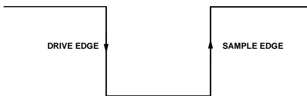
Figure 38. SPI Mode 3 SCLK Edges
