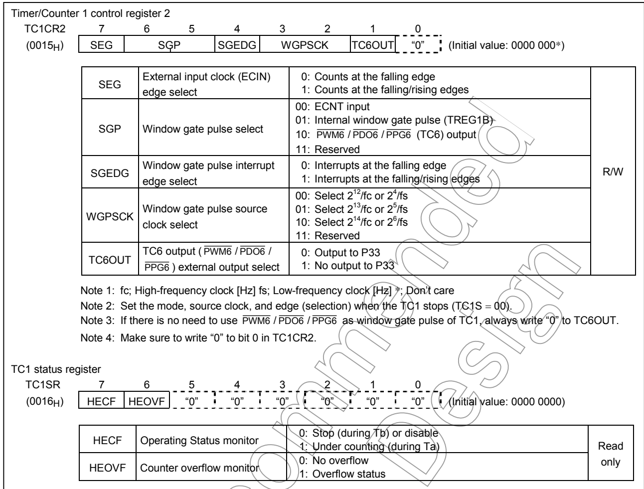
Figure 2.7.3 Control register of the TC1/status register
