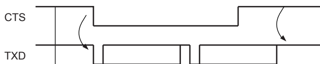
Figure 44-27. Transmitter Behavior when Operating with Hardware Handshaking
