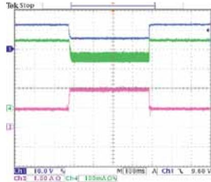
Fig.6 shows the LED current during an input step change from 13.5 to 42V and back to 13.5V (similar to a clamped load dump). It can be seen that the LED current drops briefly when the input voltage jumps, but there are no overshoots.
