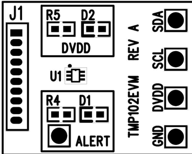
Figure 24. TMP102EVM PCB Top Layer (Component Side)
