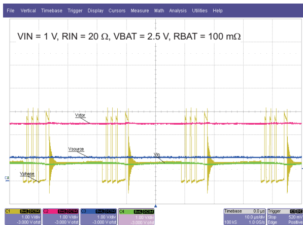
Figure 18. Example of PFM Switching Converter Waveform
