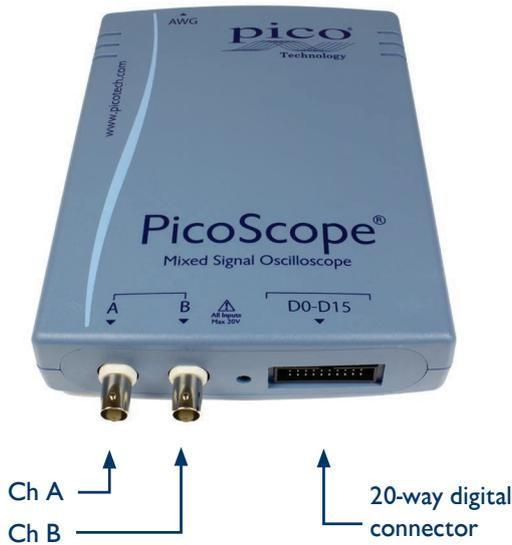
The front panel of the PicoScope 2205 MSO has two BNC analog input channels and a 20-way connector with 16 digital inputs.
