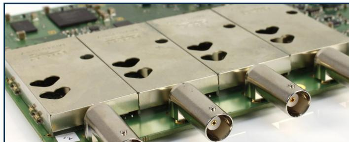
Careful front-end design and shielding reduces noise, crosstalk and harmonic distortion. Years of oscilloscope experience leads to improved pulse response and bandwidth flatness.
