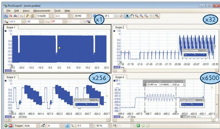
The deep memory can be segmented to store multiple waveforms, and has navigation tools allowing you to review up to 10,000 previous entries. No longer will you see a glitch on the screen only for it to vanish before you stop the scope. A mask can be applied to filter out waveforms of interest.
