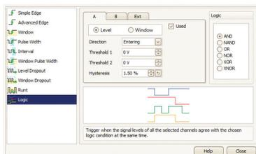
As well as the standard range of triggers found on all oscilloscopes, the PicoScope 3000 Series offers a class-leading set of advanced triggers including pulse width, windowed, dropout and logic triggers to help you capture the data you need.
