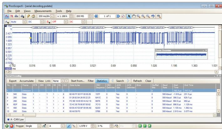
The deep-memory PicoScope 3000 Series is ideal for serial decoding as it can capture thousands of frames of uninterrupted data.
