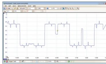
All units have a built-in function generator (sine, square, triangle, DC level) with frequency sweeping capability. Combined with the spectrum peak hold option, this makes a powerful tool for testing amplifier and filter responses.
