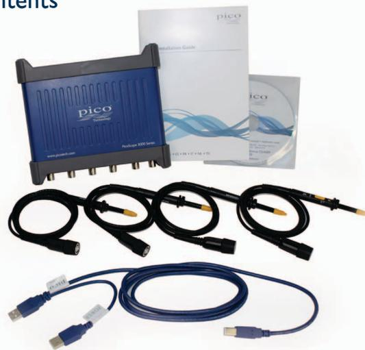
Your PicoScope 3000 Series oscilloscope kit contains the following items:
