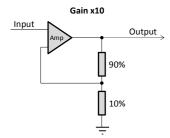
With an infinite gain the amplifier is no good to amplify audio, which is where the feedback comes in. By making one of the input a percentage of the output the gain can be fixed, which allows the output to be a copy of the input but bigger. Now when the two inputs are compared and the output is adjusted, instead of it going up or down until it reaches 0 volts or V+, it stops at the point when the two inputs match and the output is at the required voltage.
