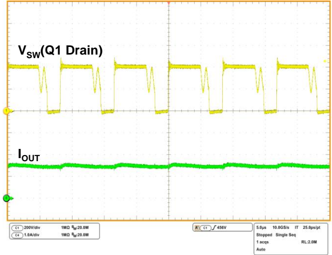
Switching Waveform V_{IN}=220V_{RMS} / 50Hz VDIM=3.3V, LED:OSW4XAHDE1E
