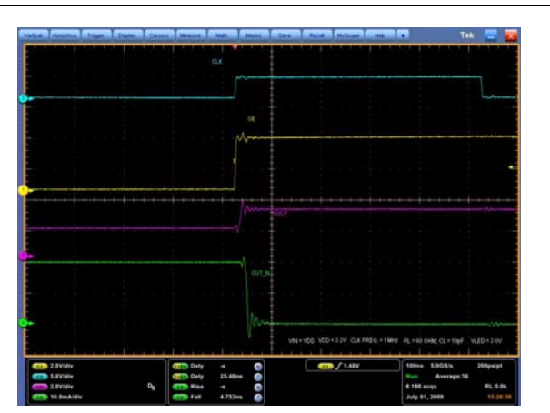
Figure 17. Turn OFF output current characteristics (2)
