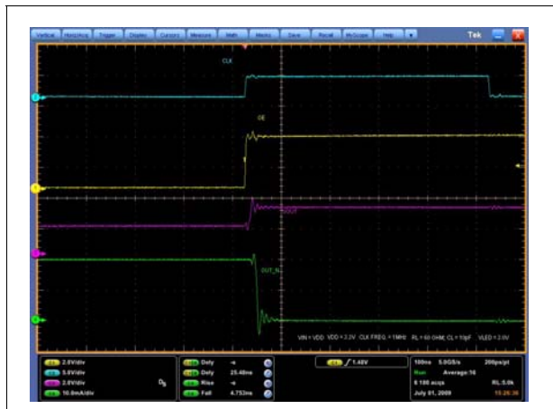
Figure 16. Turn ON output current characteristics (1)
