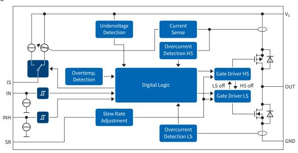
The BTN8982TA provides a cost optimized solution for protected high current PWM motor drives with very low board space consumption.
