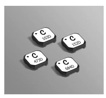
The LPD5010 coupled miniature shielded inductors are mere 1 mm high and 5 mm square. They are ideal for use in a variety of circuits including flyback, multi-output buck, SEPIC and Zeta.
