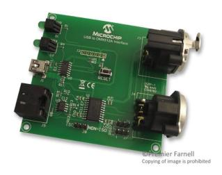
The Lighting Communications Development Platform provides a universal lighting development platform for the creation of communications enabled lighting applications. The platform consists of a main board and various communications interface adapters to support in the development of DALI, DMX512A, as well as future protocols.
