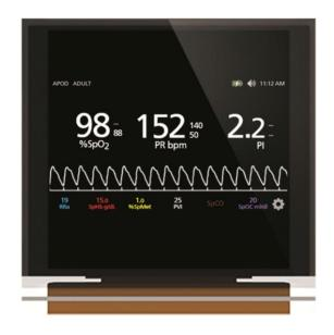
The 4DOLED-282815 is a 1.5" 128x128 pixel resolution 262K colour Passive Matrix OLED display. This OLED is the same display used in the microOLED range of modules. It allows a very cost effective means of adding a full colour small display to any product or your next microcontroller project.
