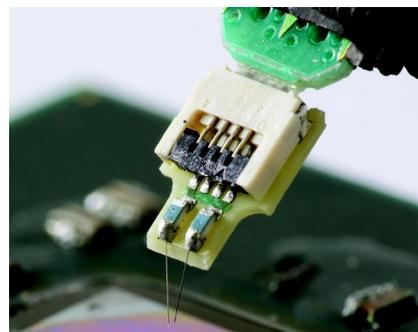
**N2887A InfiniiMax Soft touch Pro Probe Adapter** adapts from the Keysight Pro Series (36 ch) Soft touch connectorless logic analyzer foot print to the Keysight InfiniiMax I & II series probe amplifier input connectors
