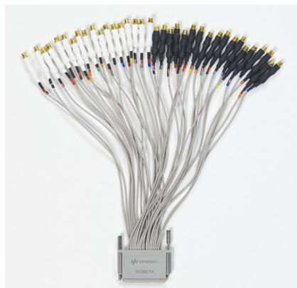
**N2888A InfiniiMax Soft touch half-channel Probe Adapter** adapts from the Keysight half-channel (18 ch) Soft touch connectorless logic analyzer foot print to the Keysight InfiniiMax I & II series probe amplifier input connectors
