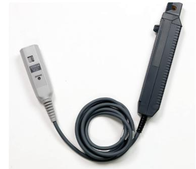
N2893A 100-MHz current probe with AutoProbe interface
