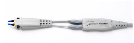
For high-speed differential or single-ended probing in embedded designs, the InfiniiMax 1130A Series differential probe amplifiers are perfect complements to the Infiniium 600 MHz – 6 GHz oscilloscopes. Its extremely low input capacitance, flat frequency response and the patented resistor probe tip technology provide ultra low loading of the DUT and superior signal fidelity.
