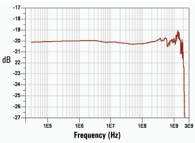
Frequency response of N2796A (V<sub>out</sub>/V<sub>in</sub>)
