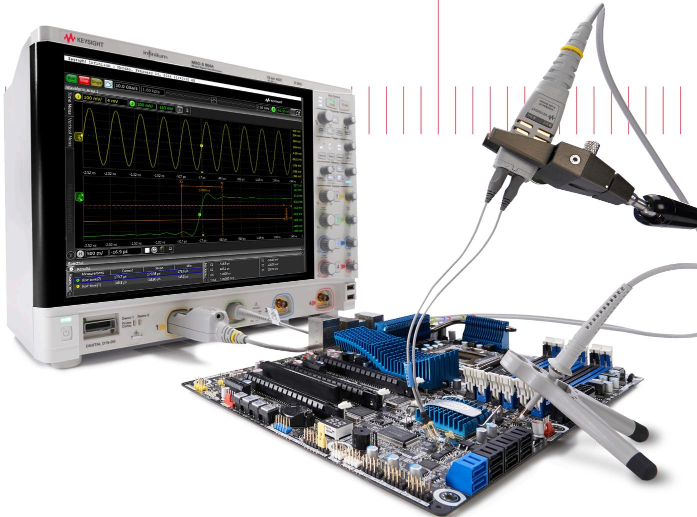
To get the most out of your Infiniium oscilloscope, you need the right probes and accessories for your particular applications. Whether you need the high bandwidth and low loading of an active probe, an easy way to connect to surface mount ICs, or a passive probe to measure high voltages, there's a wide selection of high-quality probes and accessories for your Infiniium oscilloscope.
