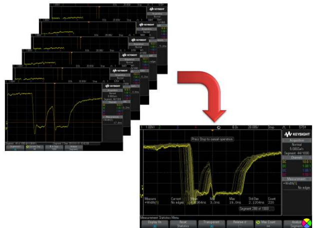
Capture 1000 very infrequent glitches over 100 seconds using segmented memory, then run inter-segment measurement and overlay analysis on the 1000 segments.
