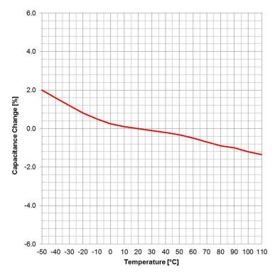
Test Equipment: E4991A or equivalent
