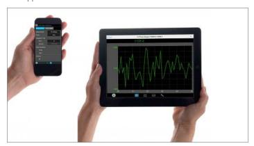
BenchVue Mobile is a mobile app that you can install on an Android or Apple iOS device to control BenchVue bench applications running on your Windows computer. BenchVue Mobile connects to your computer as a client, and requires that your mobile device and computer be connected to the same local network or intranet (behind the same corporate firewall). This network connection can be made via a WiFi connection inside your work location or externally through a VPN connection.
