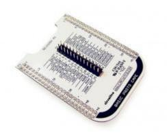
The Basic Proto Cape is designed to break out 26 signals from the expansion headers of the BeagleBone Black including GPIO, I2C, SPI, UART, PWM, analog inputs, +5V, +3V3, and +1.8V (analog). These signals can be accessed via a 26-pin male header.
