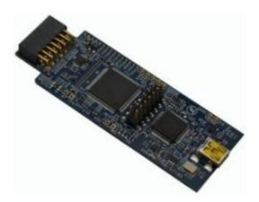
XDS100V3 is the third version developed from xds100. It is compliant with IEEE 1149.7 and implements emulation and debugging of Tl's chips through a standard 14-pin JTAG interface.
