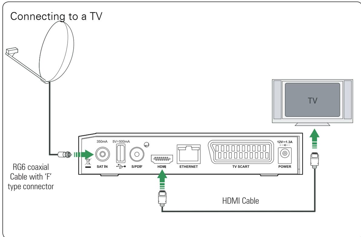
Connect a RG6 co-axial cable fitted with 'F' a type connector from your satellite dish to the 'SAT IN' socket on the back panel of your digital box.
