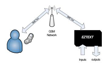
EZTEXT is a self contained two way Remote Control System which provides two changeover contact Switching outputs and two 'no volt' switched inputs.
