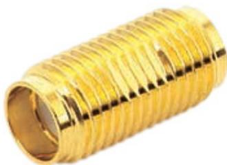
SMA connectors are semi-precision, subminiature devices that provide repeatable electrical performance from DC to 12.4GHz with flexible cable. Semi-rigid cabling extends the frequency range of the device to 18GHz. These devices offer broadband performance with low reflection and constant 50Ω impedance. These properties, along with minimum attenuation and low VSWR have made the SMA extremely popular in the microwave community.
