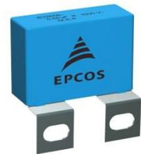
The MKP B32656S\* to B32658S\* series is distinguished by its high pulse strength and reliability of the contacts. In addition, these components offer extremely low ESL values. The series comprises 17 terminal configurations of tin-plated copper straps with a hole spacing ranging from 19.5 mm to 63 mm. These snubber capacitors now cover a voltage range from 850 V DC to 2000 V DC and a capacitance range from 68 nF to 5.6  $\mu$ F. All types are designed for temperatures of up to +110 °C.
