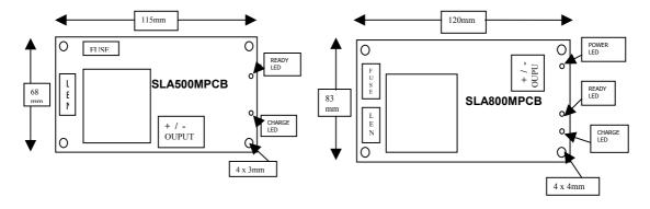
**Note:** The card must be mounted to provide adequate insulation requirements for the application. Maximum earthed metalwork screw heads/ washers etc. ≤5mm diameter without additional insulation. Attention should be paid to allowing sufficient cooling/ ventilation around the pcb in all eventualities of operation. The heatsink can get very hot.
