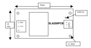
Note: The card must be mounted to provide adequate insulation requirements for the application. Attention should be paid to allowing sufficient cooling/ ventilation around the pcb in all eventualities of operation. The heatsink can get very hot.
