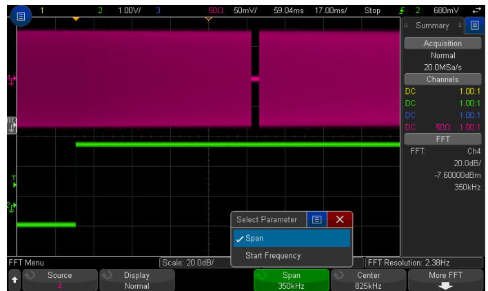
Figure 1. Enable clock (green) and oscillator output (fuchsia) options to set spectrum parameters.
