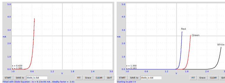
Figure 4.3: I-V characteristic of (a) Silicon diode (b) several LEDs
