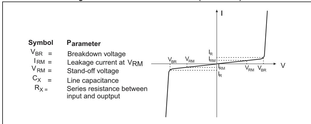
**Table 3. Electrical characteristics ( $T_{amb} = 25\text{ }^{\circ}\text{C}$ )**
