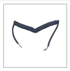
Heavy-duty cord is ideal for many applications including PA and two-way radio. Tough outer jacket is 1/4" diameter with 7/8" outside diameter coil. Contains five 24 gauge conductors plus bare shield around one. Cotton filament reinforced. Black.
