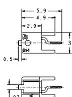
2 position mini hermaphroditic wire to board lead assembly
