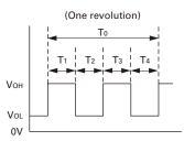
$T_{1\sim 4} = (1/4) T_0 = 60/4N \text{ (sec)}$
