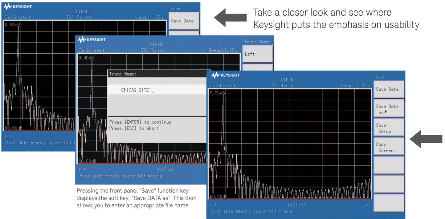
Pressing the front panel "Save" function key displays the soft key, "Save DATA as". This then allows you to enter an appropriate file name.
