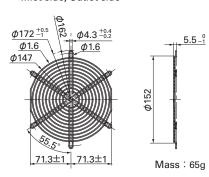
For the finger guard Model: 109-319J, fix the finger guard to four holes as shown in the diagram.
