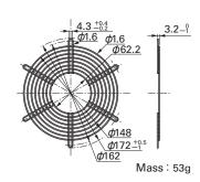
For the finger guard Model: 109-319E, 109-319H, 109-320, fix the finger guard to two holes as shown in the diagram. Do not fix it to any other holes.
