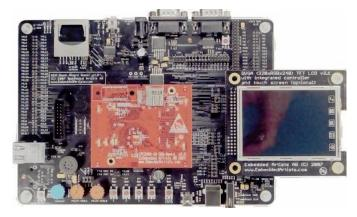
The Keil MCB2100 Evaluation Board introduces you to the NXP (founded by Philips) LPC2129 family of ARM processor-based devices. The MCB2100 allows you to quickly create and test programs for this advanced architecture.
