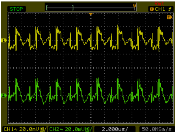
Figure 57: AXA00CC18-L Ripple and Noise Measurement Vin = 24Vdc Load: Io = ±0.67 A Ch 1: Vo1 Ch 2: Vo2
