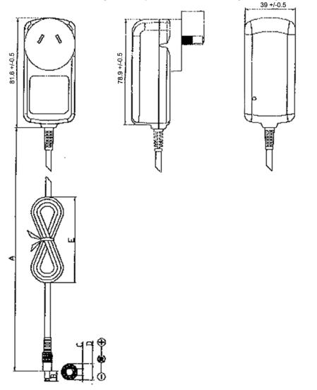
Mechanical Dimensions(Unit: mm) , Tolerance Of unspecified parts:±1mm
