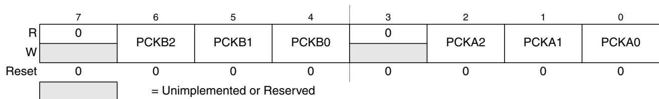
Figure 13-6. PWM Prescale Clock Select Register (PWMPRCLK)
