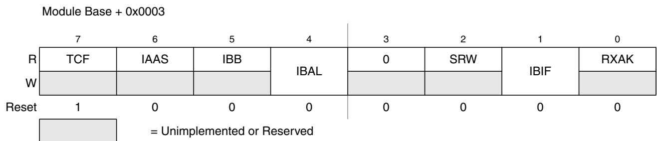
Figure 16-7. IIC Bus Status Register (IBSR)
