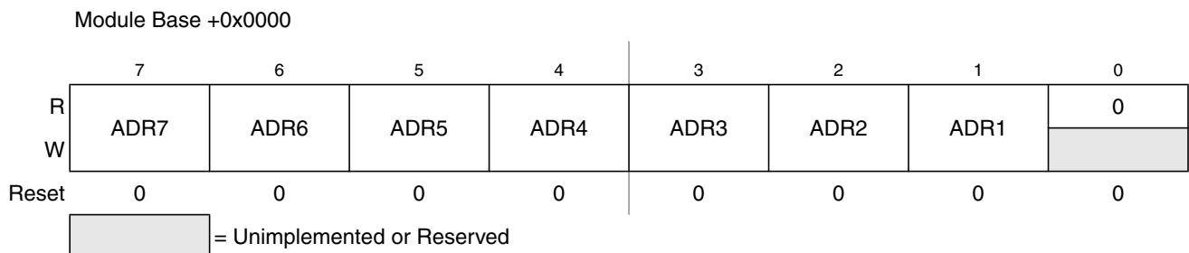
Figure 16-3. IIC Bus Address Register (IBAD)
