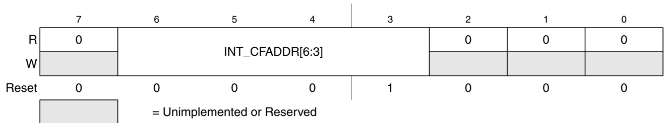
Figure 5-4. Interrupt Configuration Address Register (INT_CFADDR)
