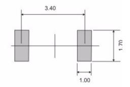
Holder Style Mode Adjustment Tolerance Operating Temp. Range Load Capacitance ESR Marking SX420A Fundamental ± 20PPM at 25°C -40°C to +85°C 6.0 pF 70000 Ohm STD
