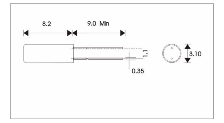
Holder Style Mode Adjustment Tolerance Temperature Stability Operating Temp. Range Load Capacitance ESR Static Capacitance (C0) Ageing Marking 3x8 Cyl Fundamental ± 20PPM at 25°C ± -.042 PPM -40°C to +85°C 12.5 pF 35K Max Ohm Unspecified pF +/-5ppm 1st Year Max Mark Std
