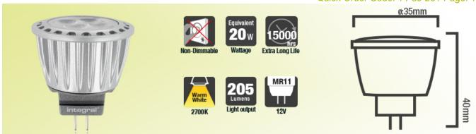
This 3.7W retro-fit Integral LED MR11 delivers brightness similar to a 20W halogen bulb, in warm light. It features quad high output Nichia LEDs, an anti-glare refractor, all finished with a diecast aluminium and plastic thermally efficient body. The ideal lamp for commercial and home use.
