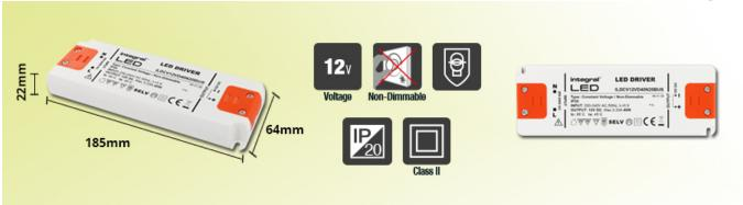
The Integral 50W constant voltage LED driver operates 200-240VAC input range. The LED driver provides 12V constant voltage and up to 4.17A of output current for a 50W maximum output power. Integral LED drivers deliver high reliability and efficiency >= 85% and are fully compatible with 12V constant voltage LED lighting systems. The LED driver features an IP20 rated casing, ideal for indoor use.
