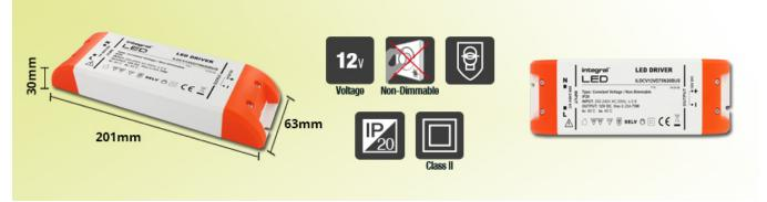
The Integral 75W constant voltage LED driver operates 200-240VAC input range. The LED driver provides 12V constant voltage and up to 6.25A of output current for a 75W maximum output power. Integral LED drivers deliver high reliability and efficiency >= 85% and are fully compatible with 12V constant voltage LED lighting systems. The LED driver features an IP20 rated casing, ideal for indoor use.
