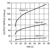
Figure 8. Output Voltage Ripple
