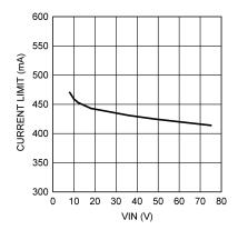
Figure 10. Current Limit vs Input Voltage
