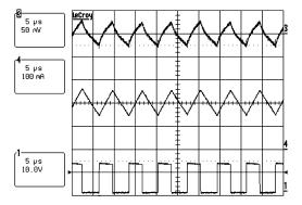
Trace 1 = SW Pin Trace 3 =  $V_{OUT}$ Trace 4 = Inductor Current
