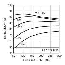
Figure 6. Efficiency vs Load Current
