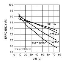
Figure 7. Efficiency vs Input Voltage
