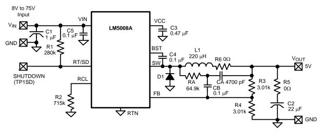
Figure 4. Minimum Output Ripple Configuration
