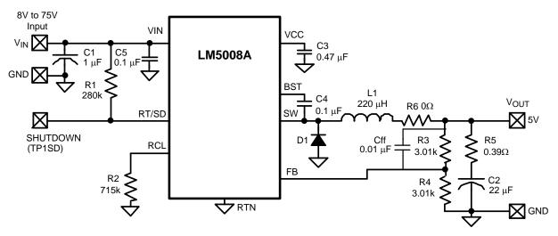
Figure 3. Intermediate Ripple Configuration
