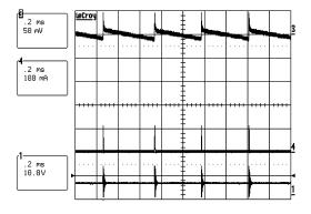
$\begin{aligned} &\text{Trace 1} = \text{SW Pin} \\ &\text{Trace 3} = \text{V}_{\text{OUT}} \\ &\text{Trace 4} = \text{Inductor Current} \\ &\text{Vin} = \text{12V, lout} = \text{0 mA} \end{aligned}$
