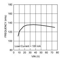
Figure 9. Switching Frequency vs. Input Voltage
