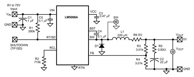
Figure 5. Complete Evaluation Board Schematic (As Supplied)
