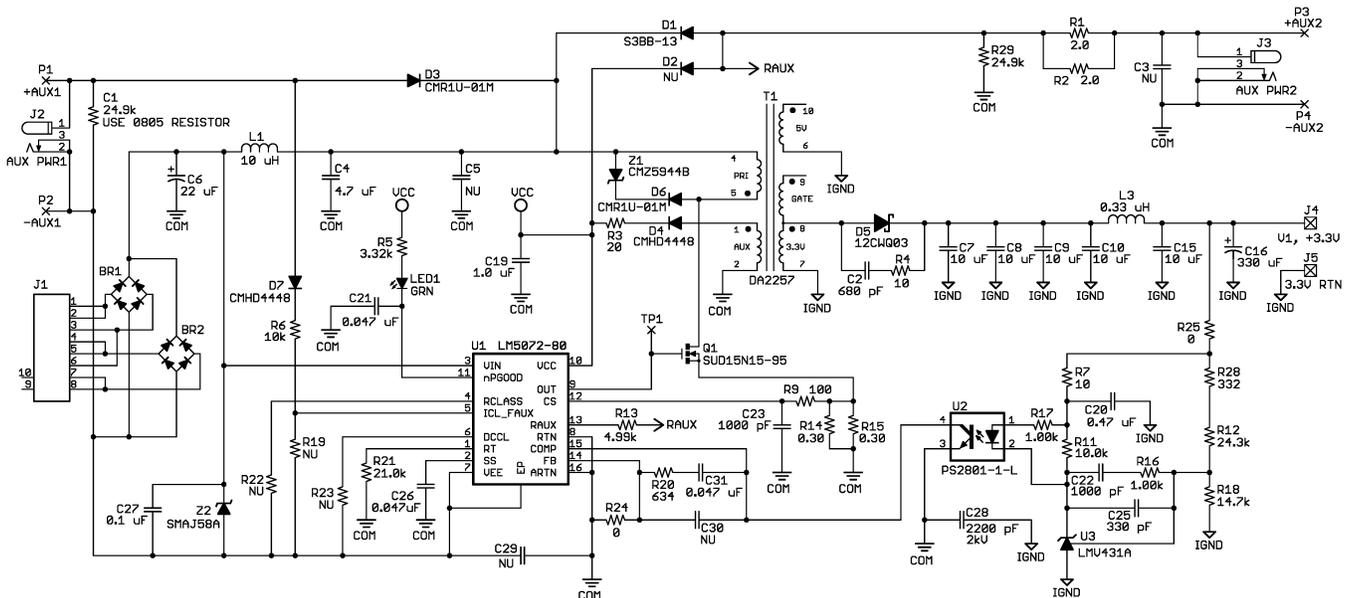
Figure 1. Schematic of the LM5072 Evaluation Board
