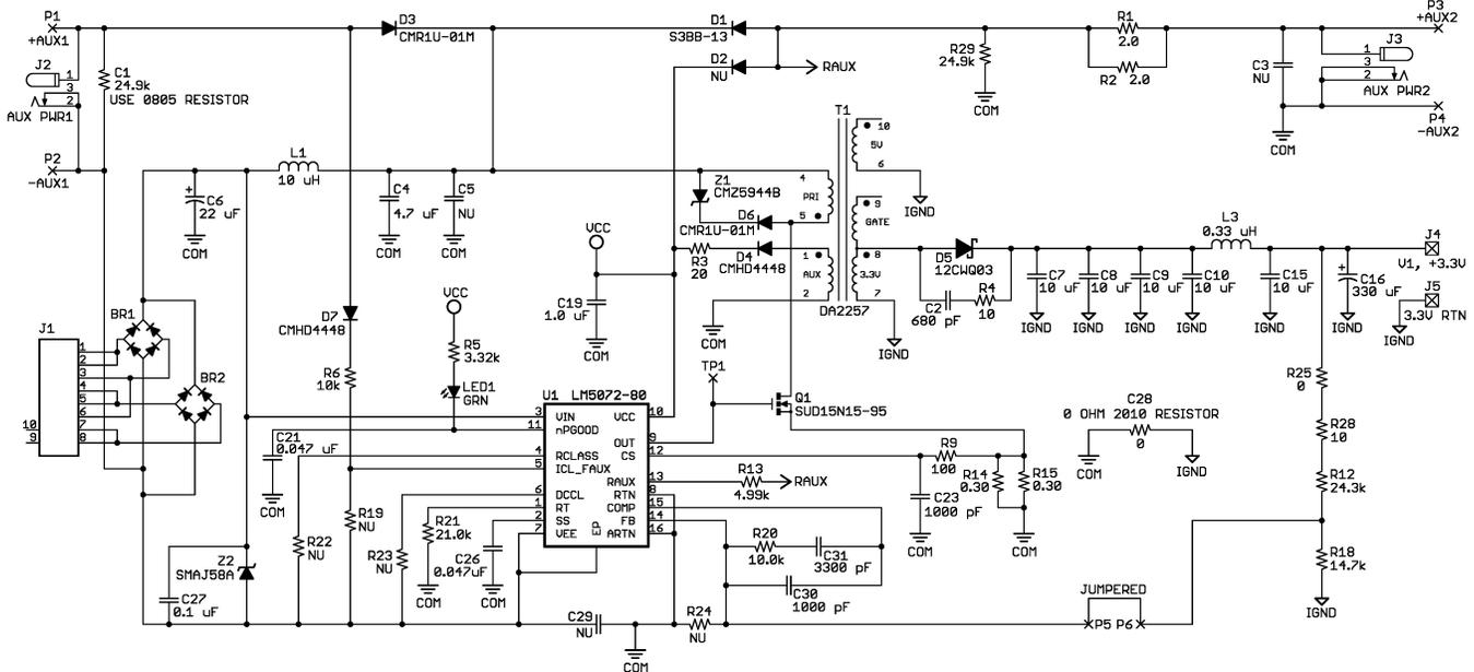
Figure 16. The Schematic for Non-Isolated Output
